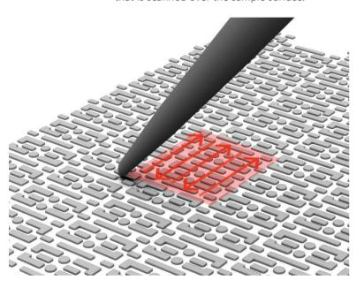
The resulting image yields information on the contacts' electrical properties. For instance, by varying the bias voltage on the tip, it is possible to selectively image n-mos or p-mos contacts.
