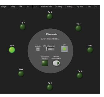
The STA offers a valuable time reduction and greatly reduces the risk of damaging the probe tip and the sample when approaching a region of interest.
