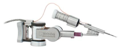
Filling the reservoir can be achieved by simply removing its cap and introducing the desired precursor material. Typical materials are: Water, Hexane, Naphthalene, Tungstenhexacarbonyl, or lodine - but pretty much anything goes! The precursors may be heated to a temperature of up to 90°C in order for them to evaporate. Using the valve's fine control, the amount of gas introduced into the chamber can be finely tuned.
