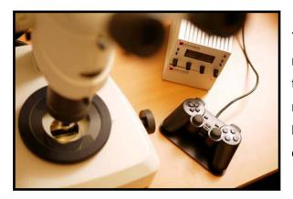
The MM3A's needle is so small it cannot be seen with the naked eye. It moves in nanometre-steps, that is moving the needle from one atom to another for uses as varied as minimal invasive surgery such as eye and ear operations, brain research in the field of life science or even working on micro computer chips or semiconductors.
