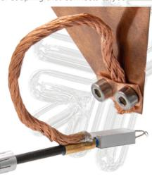
microscope's cryo shield or cryo stage. Thus, the gripper can be cooled to LN2 temperature while the MM3A-EM remains at room temperature. This greatly reduces the thermal load for your microscope's cooling system.
