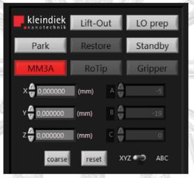
By 'talking' to the microscope, the software is able to adjust the micro-manipulator's speed of motion to match the given magnification. The software also provides true Cartesian motion using the microscope PC's mouse (for X and Y motion) as well as an additional USB jog shuttle device (for Z motion). In addition, the software is equipped with park&restore functionality and can be used to control the microgripper.
