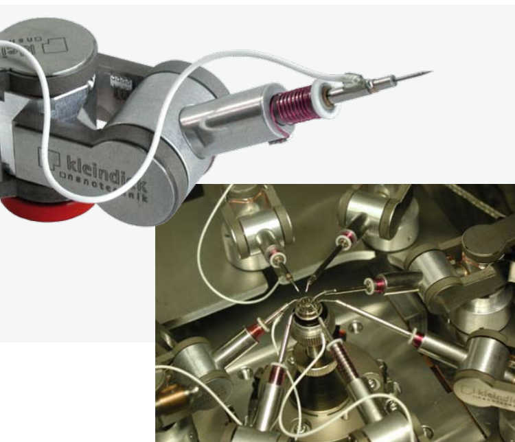
Seven MM3A-EM micromanipulators installed in an SEM - three are fitted with an LCMK-EM low-current measurement kit
