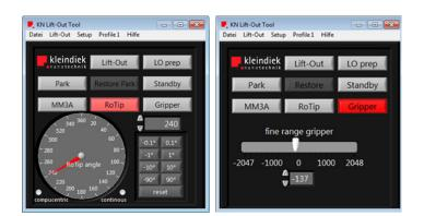
By accessing magnification and other information from the microscope's software interface, the micromanipulator's speed can be linked to the microscope's current field of view. This eliminates the need for the user to manually adjust the micromanipulator's speed.
