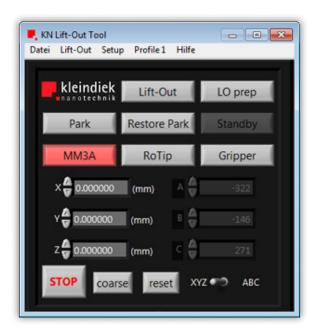
iLO provides three-dimensional control via twohanded operation – the microscope PC's mouse for X and Y movements combined with a jog dial for Z movements. Upon activating movement, the Lift Out tool becomes your mouse pointer which yields a familiar and intuitive feeling, including dynamic movement response.
