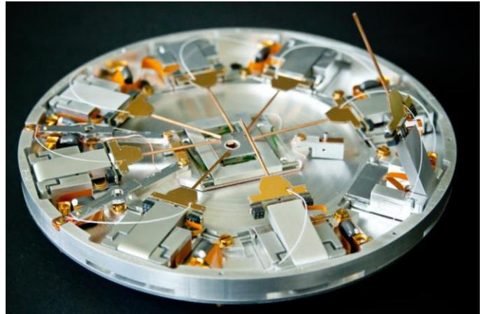
Fig. 1. Prober shuttle PS8 with 8 probes and xyz substage (14 cm diameter, 1 cm height)
